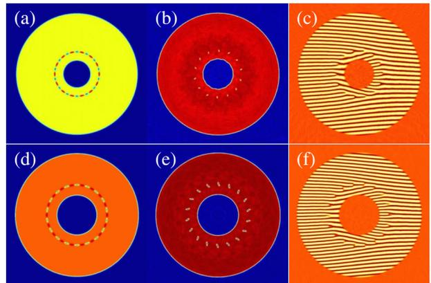
FIG. 5 (color online). Numerical simulation of the propagation of two concentric beams with nested vortices of opposite TCs  $l = 7, -7$  (a) and  $l = 9, -9$  (d); propagation constants  $\beta/\beta_{cr} = 0.98$  and  $0.99$ ; window widths (in  $\mu\text{m}$ )  $1100$  (a)–(c) and  $1000$  (d)–(f); and propagation distances (in mm)  $z = 0$  and  $10$ . Images (c) and (f) correspond to the interference patterns of (b) and (e) with a slightly tilted plane wave.
