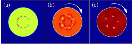
FIG. 3 (color online). Numerical simulation of the propagation of two laser beams with nested vortices of TCs  $l = 0$  and  $5$ , with propagation constants  $\beta = 0.984\beta_{cr}$  and  $\beta = 0.99\beta_{cr}$ . The outer beam has been displaced  $2 \mu\text{m}$  in the  $x$  axis. The window width is  $500 \mu\text{m}$ . The propagation distances (in mm) are  $z = 0$ ,  $0.2$ , and  $30$ .
