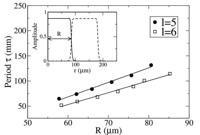
FIG. 2. Period of rotation of the vortex lattice versus internal radius of the outer beam  $R$ , considering the inner beam nodeless and the outer beam with TC  $l = 5$  and  $l = 6$ , respectively. This period represents the propagation distance  $z$  at which the angle of rotation of the lattice is  $2\pi$  rad. Inset: radial profiles of input beams with  $\beta = 0.99\beta_{\text{cr}}$  and  $l = 6$ .
