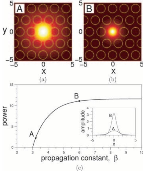
Figure 1. (a,b) Examples of stationary solutions for scalar PCF spatial solitons for  $\beta = 3.2$  and  $\beta = 6$ , and (c) power dependence of the soliton family. Points A and B in the power diagram (c) correspond to the examples (a,b), respectively. Inset: the corresponding one-dimensional profiles at  $y = 0$  for both examples.
