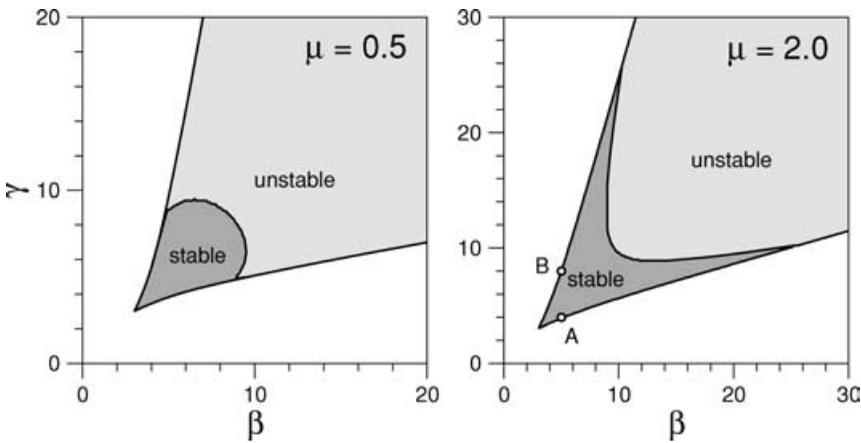
Figure 4. Existence domain for the vector solitons in PCF in the plane  $(\beta, \gamma)$ , shown at two values of the coupling parameter  $\mu$ . Labeled points correspond to two particular examples shown in Figure 3.
